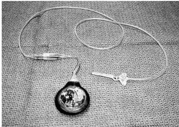
Fig 1. The phrenic nerve electrode wire is shown attached to the receiver. They are detached from one another during lead placement to facilitate passage of the male end of the electrode through the diaphragm. The long tab on the electrode can be reduced by half its length to facilitate insertion into the chest and positioning around the nerve.
